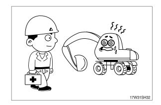
Park on a flat place and stop the engine for inspecting and repairing. Properly TAG machine is not operational. (remove start key)
